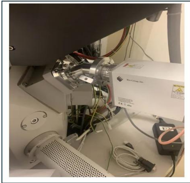
Figure 1 ibssGroup downstream ICP plasma on a NovaNano 230 SEM from ThermoFisher
